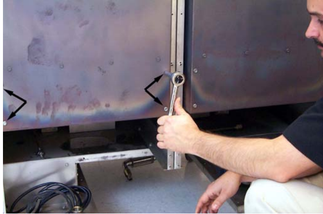
Removing bolts (arrows) securing flue to cookpot.
