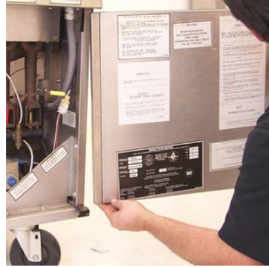
Remove door for easier access to temperature probe.
