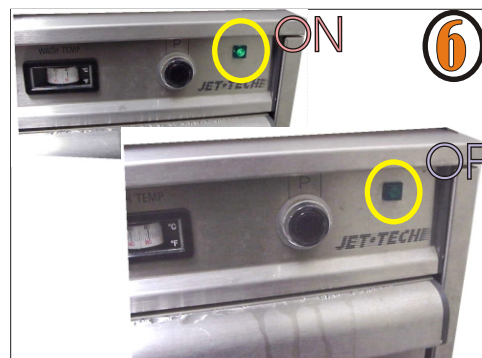
6 Wait for the green light to turn off before taking the tray out. Take tray out to let dishes air dry. Repeat from #3.
