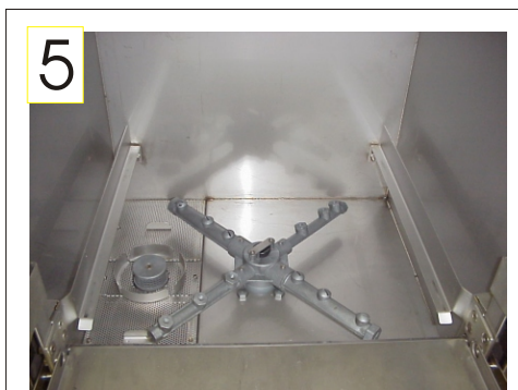
Replace all parts in the wash tank. Leave the dishwasher empty overnight and the door closed.
