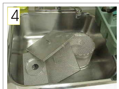
Clean the screens and wash tank of debris. Rinse wash tank.
