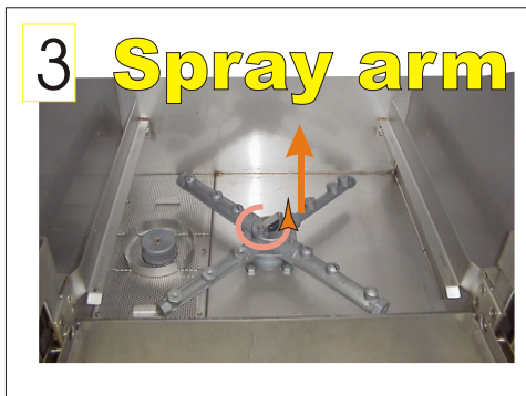
Water must all drained from the wash tank. Do not flush any dirt down the drain. Remove the spin-arm and the screens.
