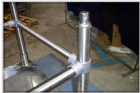
Figure 2—Cross brace set-up
