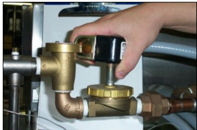
Removing the coil
