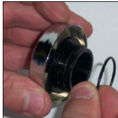
Replacing the O-ring
