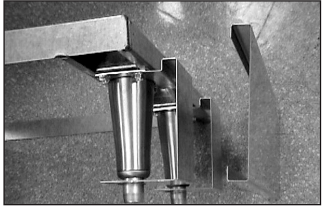
Toe plate installation.
